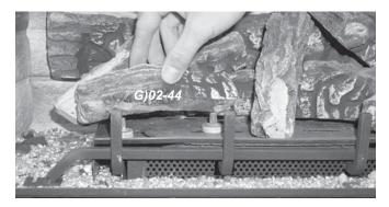
**10)** Place the embers and Rockwool on the exposed front burner tray.
